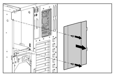
Figure 2-35. Removing the power supply cover plate
